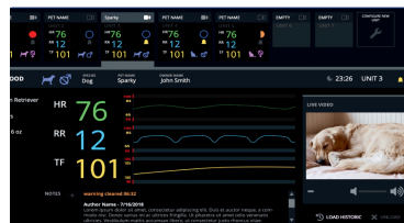
ACCESS VITALS MONITORING CONTINUOUSLY MONITORS TEMPERATURE, PULSE, AND RESPIRATION WITH LIVE VIDEO
