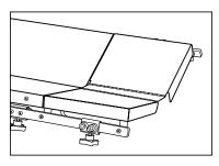
10" stainless steel table top extensions for V- top surgery tables are available. Extensions may be added to each end. Two extensions provide 20" of additional work surface length. *For 50" table only.*
