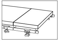
10" stainless steel table top extensions for flat-top surgery tables are available. Extensions may be added to each end. Two extensions provide 20" of additional work surface length. *For 50" table only.*
